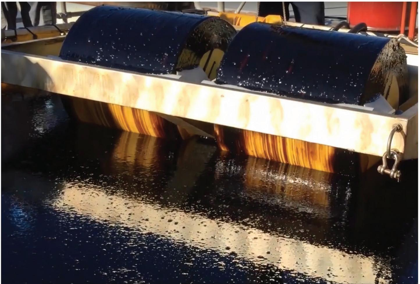
*Alaska North Slope crude oil/i-Petrogel solution is recovered by an Elastec TDS 118 oleophilic drum skimmer. The recovered oil/i-Petrogel solution contains almost no water and can be refined using regular refining processes. Overall, i-Petrogel technology potentially provides a comprehensive solution for combating crude oil spills in open waters, with dramatic reduction in environmental impacts. Photo: Courtesy Mike Chung*
