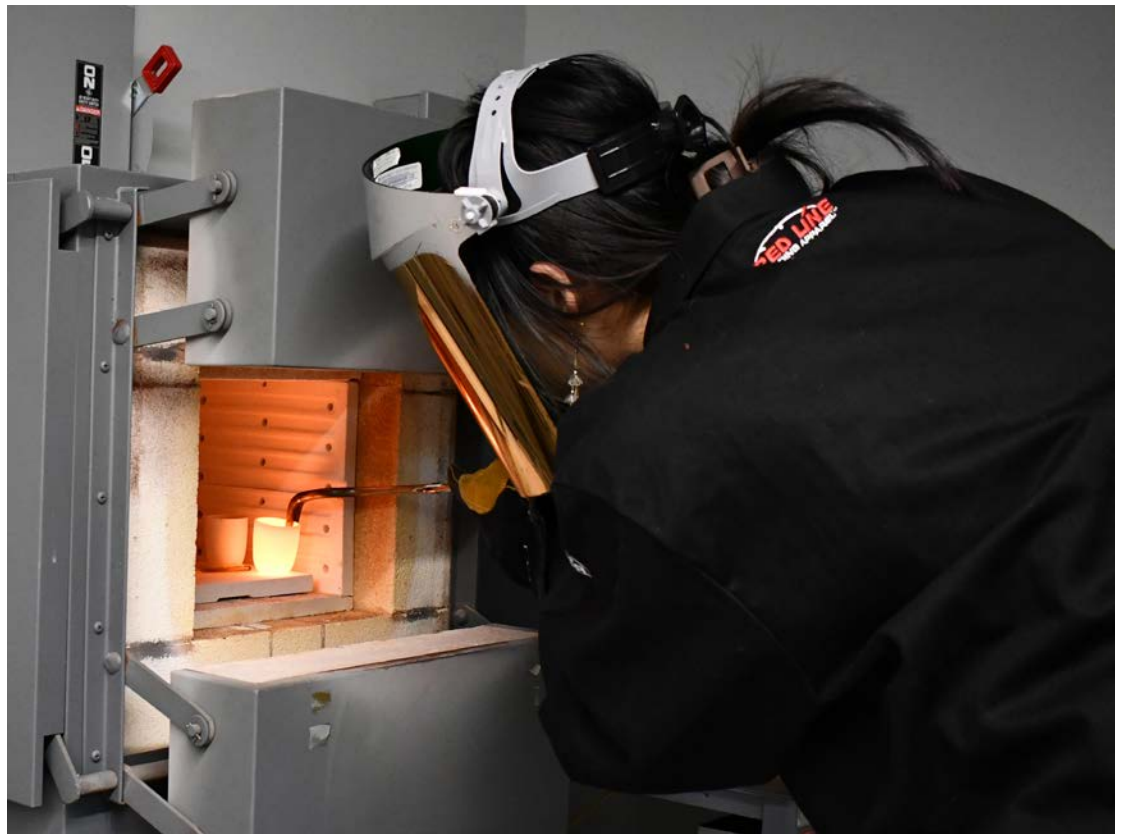
Julia Chen, an undergraduate student in materials science and engineering, places a sample of LionGlass in the annealer in Mauro’s lab.
