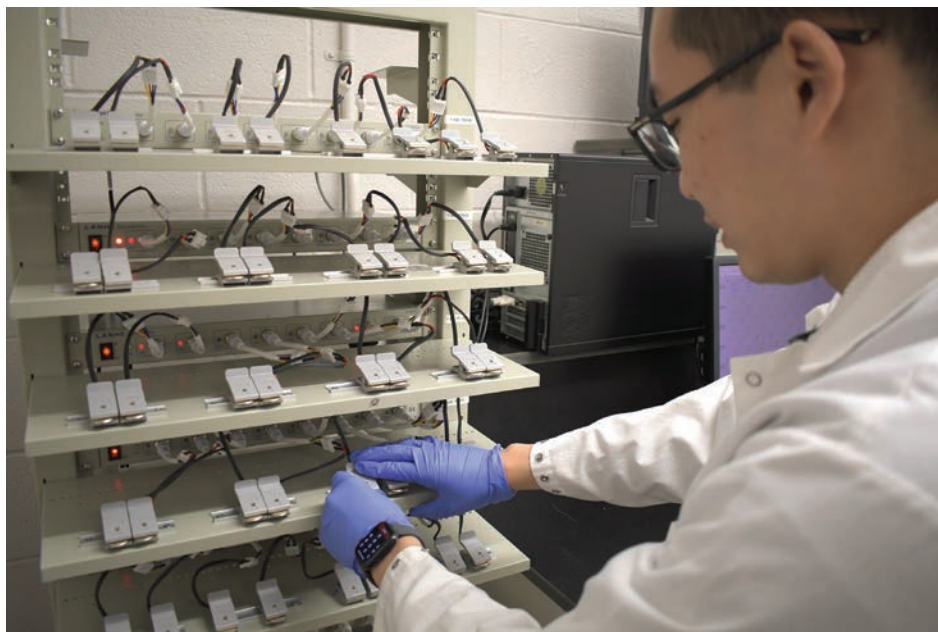
Hanrui Zhang, a graduate student in Shi's lab, tests the cycling performance of coin cell batteries.
