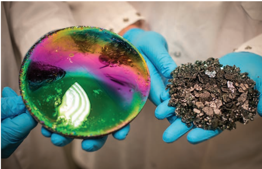
If all goes well, a colorful SiC boule is created (left), and a "crown" on the source SiC forms (right).
